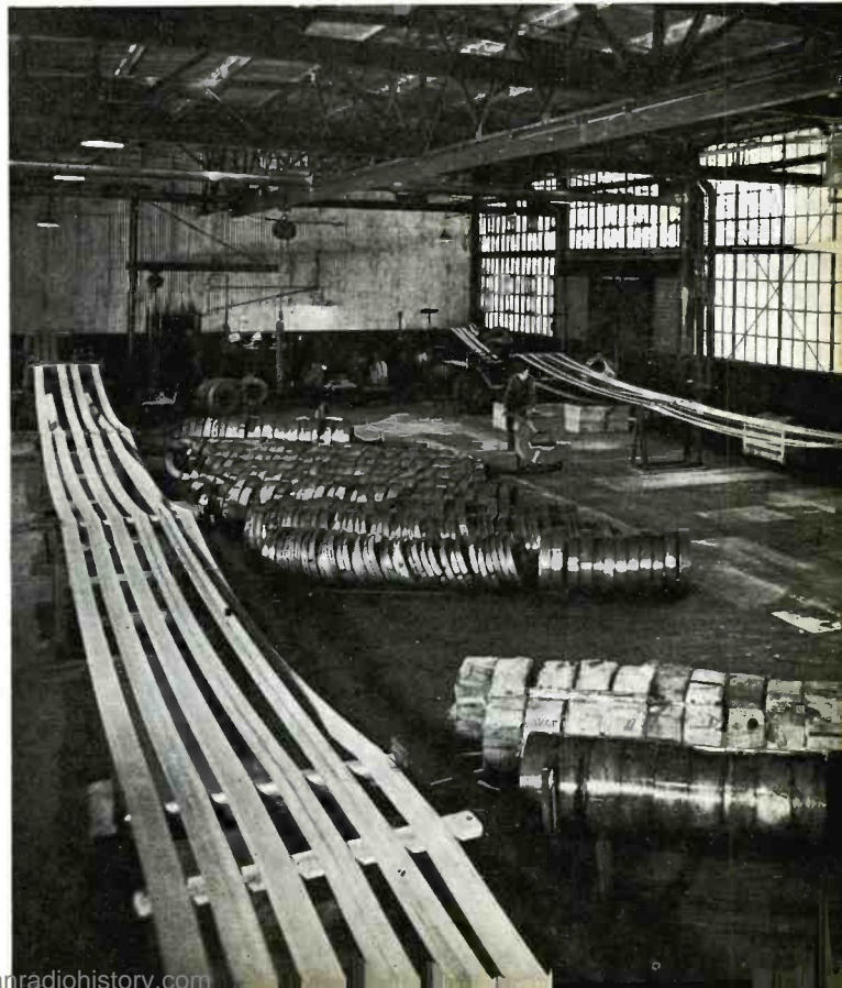
Silicon strip leaving annealing furnaces, and cooling as it travels to the coiling machines.
